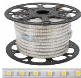
Tira de 60 LEDs/M 220VAC 50M SMD5050 IP65
